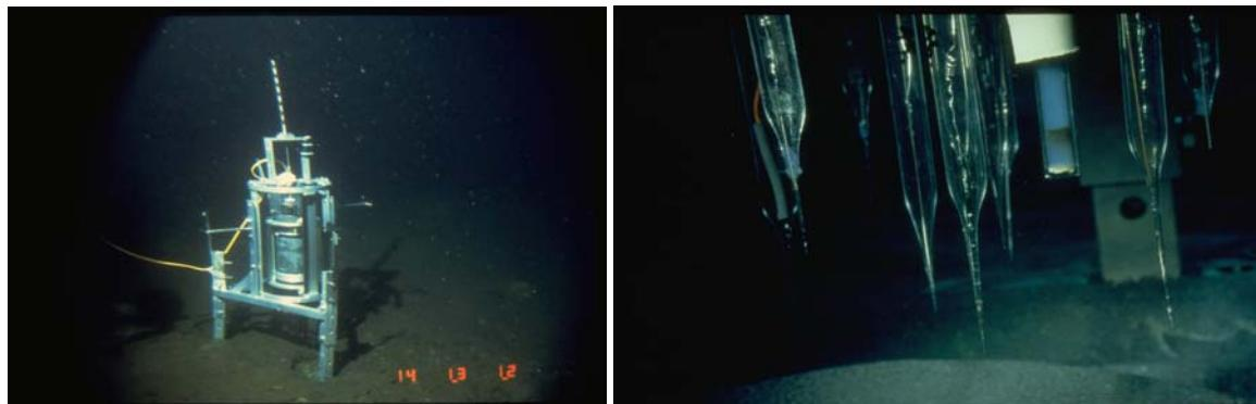
**Ultra-low oxygen measurements.** Some areas of the ocean have such a low oxygen concentration that it can be difficult to determine whether it is actually zero. With micro-sensor technologies, it is possible to construct a sensor, which can intermittently block and un-block the access of oxygen to the sensor, which allows a detection limit of  $5 \text{ nM}$  ( $1.6 \times 10^{-4} \text{ mg/l}$ ). The sensor principle will be discussed and data presented.
